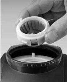
Ensure that the black adjustment ring is rotated counterclockwise as far as it will go. Replace the burr by lining up the red tab on the burr with the rectangular cutout on the black adjustment ring. Wiggle and push down firmly on the ring burr to ensure that it seats properly.
